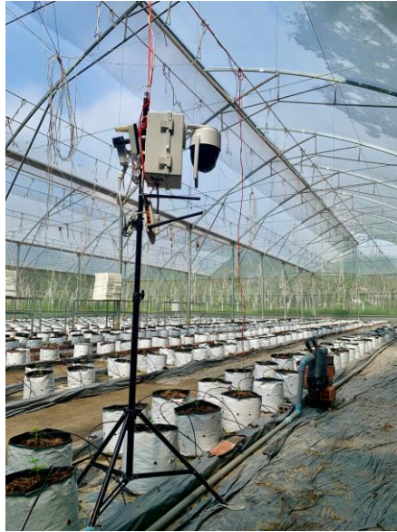
Fig.1. IoT system model for growth observation of melon at RCHAA University of Science (VNUHCM).
